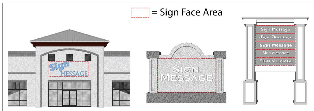
Figure 9-6: Measuring Sign Area
